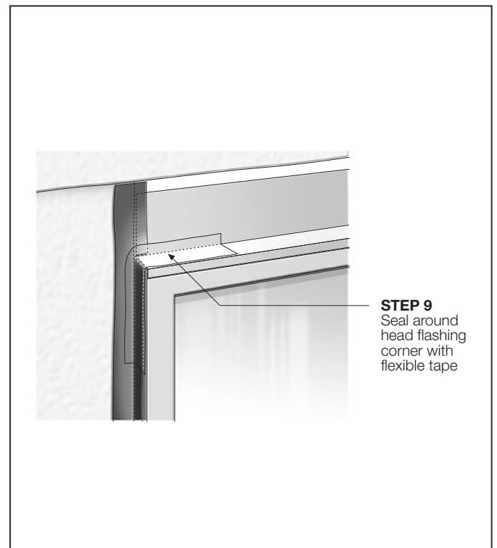
FIGURE 46 INSTALLATION OF WINDOW
